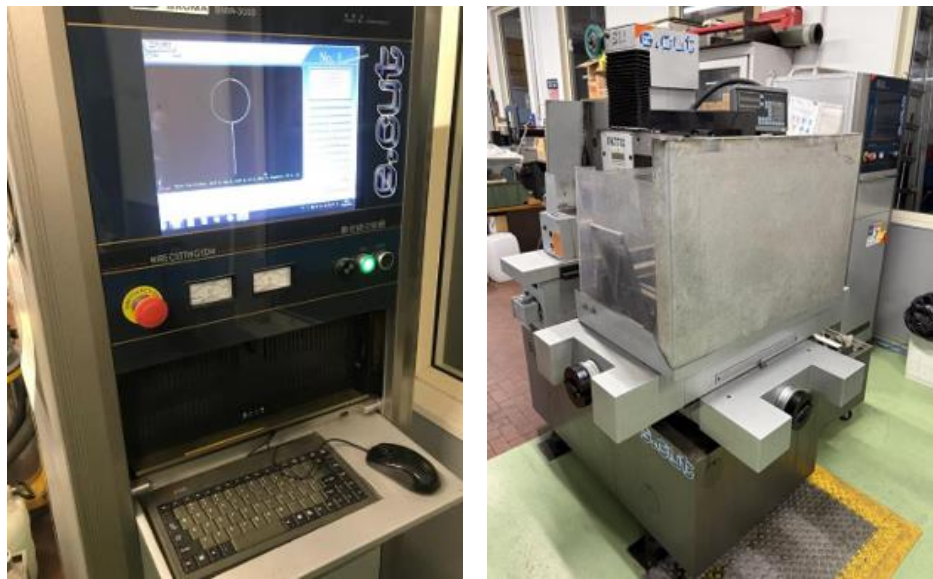
Figure 15: a) CAD Software of G.cut Machine b) G.cut W-EDM, coordinate display and cutting area
