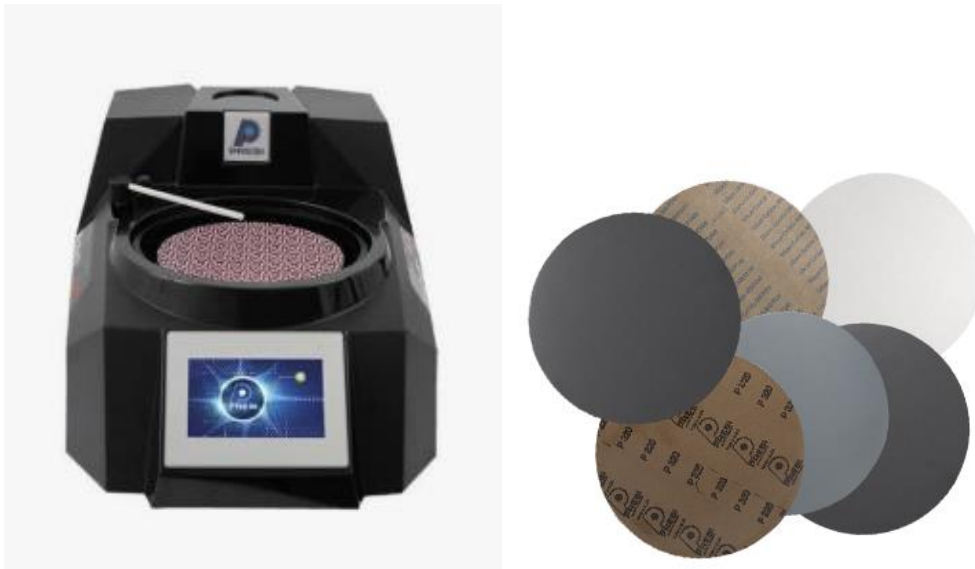
Figure 20: The Presi machine was used for the grinding and polishing of the samples. And SiC abrasive papers
